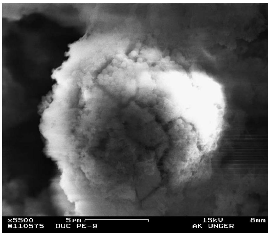
Fig. 19. SEM image of polyethylene product following polymerization with carrier 2c. Polymerization conditions: 0.5 g carrier, 5.4 mmol MAO, 4.3 μmol  $\text{Cp}_2\text{ZrCl}_2$ , 0.4 mmol TIBA, 2.5 bar ethylene, 115 mL toluene, 1 h polymerization, begun at room temperature (see Section 5).
